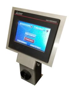
Car-wash interface which allows staff to monitor and control some of the car-wash functions and equipment
